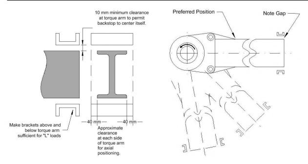
Safe backstop mounting is possible at any desired angle of the torque arm. However, mounting the backstop in a straight vertical position is not recommended. A minimum angle, approximately 5 degrees from vertical, should be maintained.
