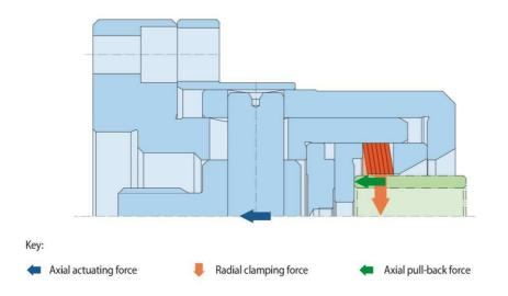
The bonded disc pack sits pre-loaded in the seating diameter of the seating body. To actuate clamping the bonded disc pack is raised to an upright position by axial actuating force. The component is centred, pressed flush against the shoulder ring and aligned. The tipping movement of the bonded disc pack converts the axial actuating foce into a radial clamping force that is up to 10 times higher.
