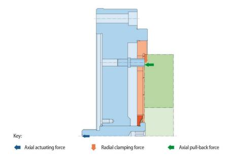
The flat element sits pre-loaded im the seating body. For clamping the flat element is elastically deformed by the axial actuation force. The component is centred, pressed against the backstop and aligned flush.
