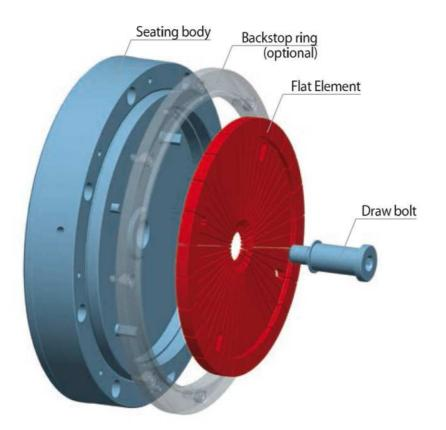
The Flat Element Flange Chuck consists of a seating body with backstop pins, a flat element and a draw bolt. A backstop ring and an sub assembly for manual clamping are also available as options. The Flat Element Flange Chuck is attached to the machine with the seating body. The clamping fix-ture is actuated by the draw bolt which is connected to the machine power actuating unit.
