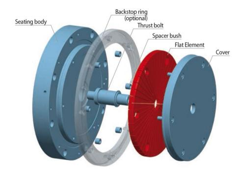
The Flat Element Flange Mandrel consists of a seating body, a thrust bolt, a set of spacer bushes, a flat element and a cover. A backstop ring and an sub assembly for hand clamping are optionally available. The Flat Element Flange Mandrel is attached to the machine with the seating body. The clamping fixture is actuated by the thrust bolt which is connected to the machine power actuating unit.
