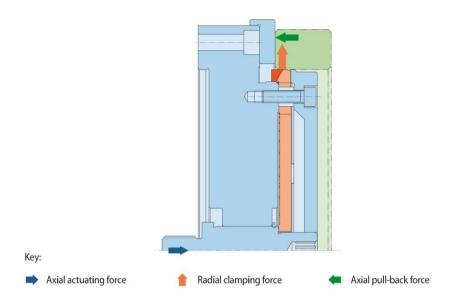
The flat element sits pre-loaded on the seating body. For clamping the flat element is elastically deformed by the axial actuation force. The component is centred, pressed against the backstop and aligned flush.
