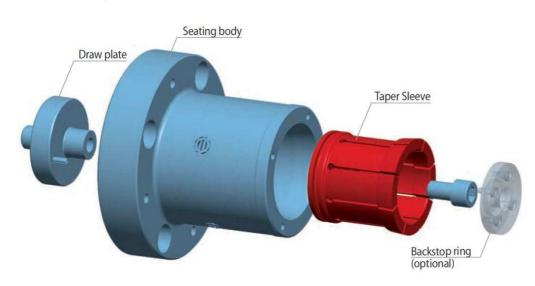
The Taper Sleeve Flange Chuck consists of a draw plate, a seating body and a taper sleeve. A plain parallel ground backstop ring and a plate with a threaded bore for hand clamping are optionally available. The Taper Sleeve Flange Chuck is attached to the machine with the seating body. The clamping fixture is actuated by the draw plate, which is connected to the machine power actuating unit.
