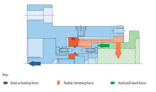
For clamping the taper sleeve is pulled against the seating body. The component is centred, pressed against the backstop and aligned flush.
