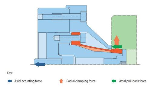
For clamping the seating body is pulled against the seating body. The component is centred, pressed against the backstop and aligned flush.
