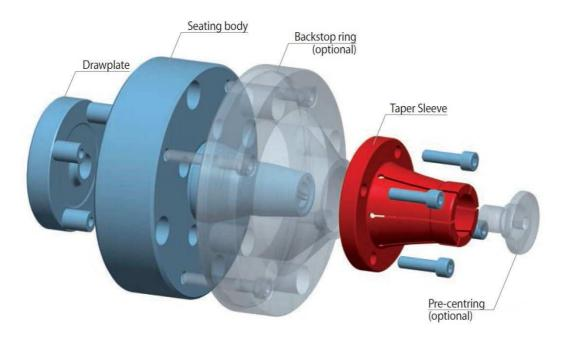
The Taper Sleeve Flange Mandrel consists of a draw plate, a seating body and a taper sleeve. A backstop ring and a pre-centring are optionally available. The Taper Sleeve Flange Mandrel is attached to the machine with the seating body. The clamping fixture is actuated by the draw plate, which is connected to the machine power actuating unit.
