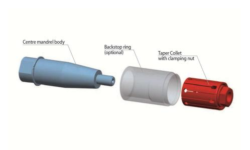
The Taper Collet Centre Mandrel BKDI consists of a centre mandrel body and a taper collet with a clamping nut. A plain ground backstop ring is also available as an option. The Taper Collet Centre Mandrel is mounted between the centring tips. The taper collet is activated by turning the clamping nut.
