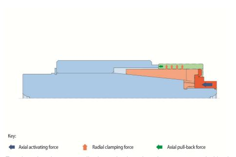
For clamping the taper collet is pushed against the centre mandrel body. The component is centred, pressed against the optional backstop ring and aligned flush.
