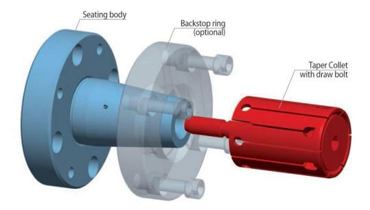
The Taper Collet Flange Mandrel consists of a seating body and a taper collet with draw bolt. Taper collets with hexagon head (series BAD) or pre-centring (series BVD)., A sub asse,bly screwplate for hand actuation is optionally available. A backstop ring is individually design according to the component. The backstop ring is normally manufactured by ths customer.
