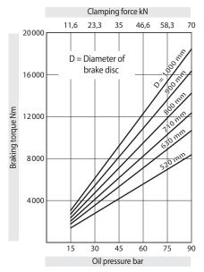
The braking torques shown in the diagram are based on a theoretical friction coefficient of 0,3.
