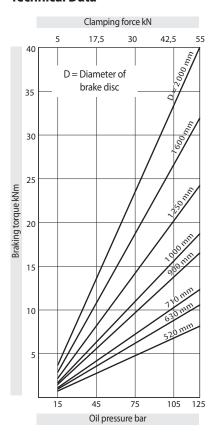
The braking torques shown in the diagram are based on a theoretical friction coefficient of 0,4.
