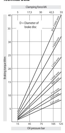
Oil pressure: min. 15 bar max. 125 bar
