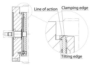
Fig. 8 Flat mandrel clamping element
