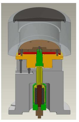
Fig. 21 Flat-mandrel clamping element with hydraulic clamping chuck for million of a large planetary pinion, power actuated. 3-D view
