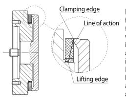
Fig. 7 disc clamping element
