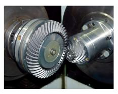
Fig. 14.2 Clamping mandrel for automotive crown gear lapping and testing
