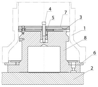
Fig. 19 Flat mandrel on machine table for transmission bell housing
