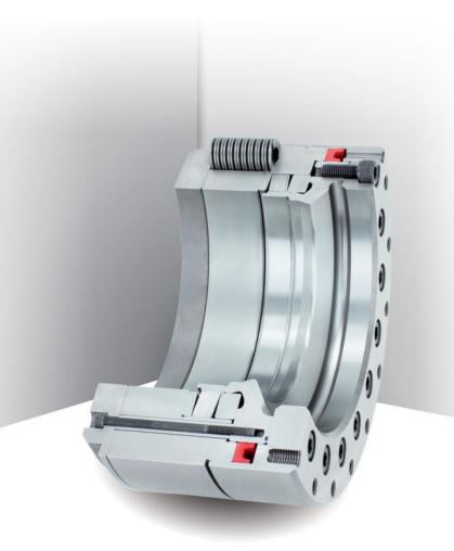
ment. This purely mechanical action ensures a fully anti-twist, all round clamping of the kingpin of the positioning axis. The clamping is quickly released by applying 115 bar of hydraulic pressure to the clamping coupling. This immediately frees the positioning axis of the rotary/swivel table again for the approach into the next angle setting. The new high-precision solution from RINGSPANN thus also supports quick changes between different angle settings of a machining process.
