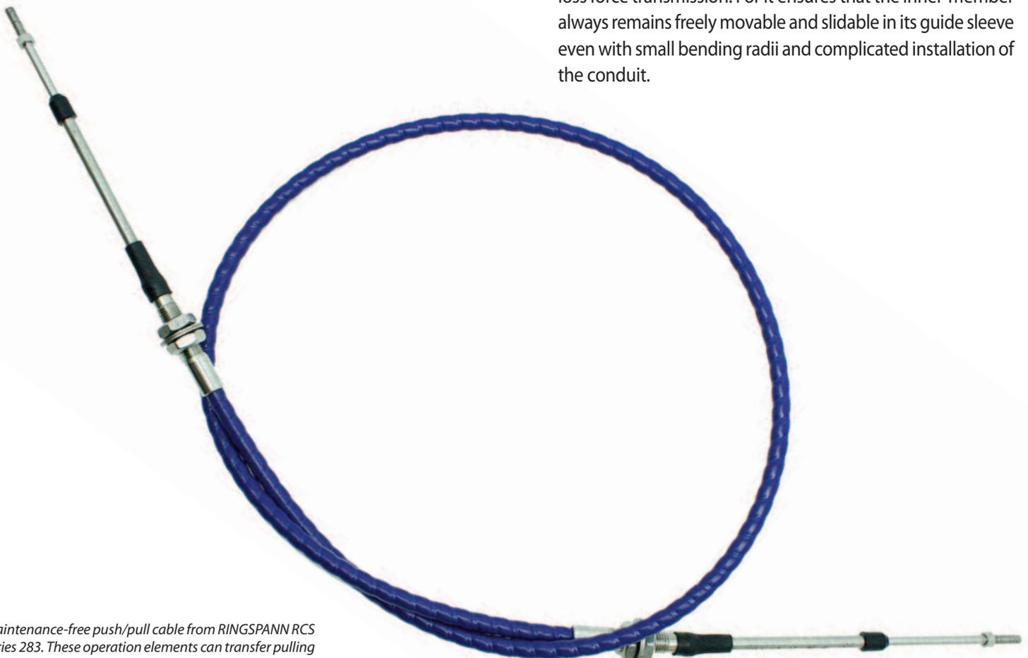
*Maintenance-free push/pull cable from RINGSPANN RCS series 283. These operation elements can transfer pulling forces of up to 4500 N and pushing forces of up to 3150 N. (Image: RINGSPANN RCS)*
